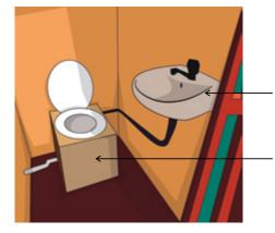
Hand washbasin is directly connected to the micro flush seat; wastewater is re-used as water seal and flush water for the next user
