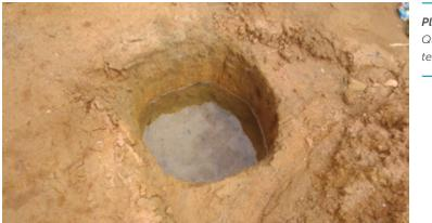
**Plate 5:** Quick waterlogging test
