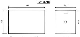
Top cover slab type 1 with 8mm reinf. rod of 100mm intervals at each way, laid on a 25mm x 25mm welded wire mesh with a thickness of 40mm concrete in a mix ratio of 1:2:4 Qty. 1no.
