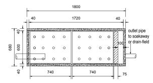
Digester made with reinf. conc. slabs and slabs with holes Bulking material not shown for clarity
