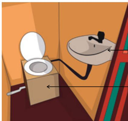
Hand washbasin is directly connected to the micro flush seat; wastewater is re-used as water seal and flush water for the next user
