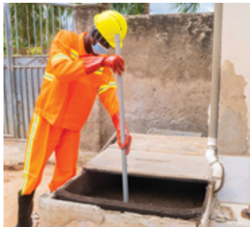
Figure 6: Dipstick being inserted in sludge to check the moisture content
