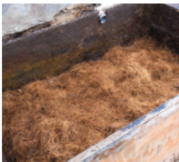
Figure 13: Placing bulking material into the biodigester
